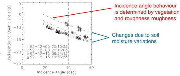
ERS Scatterometer measurements
